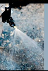
The Trilogy Defense system features a spray tube that applies liquid directly to the granular material as it enters the pre-wet mixing chamber or nozzles that can spray liquid brine directly on the surface for treatment.
