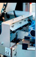
A manual lever on the pump box allows the operator to easily switch between pre-wet or direct liquid application mode when the accessory system is active.
